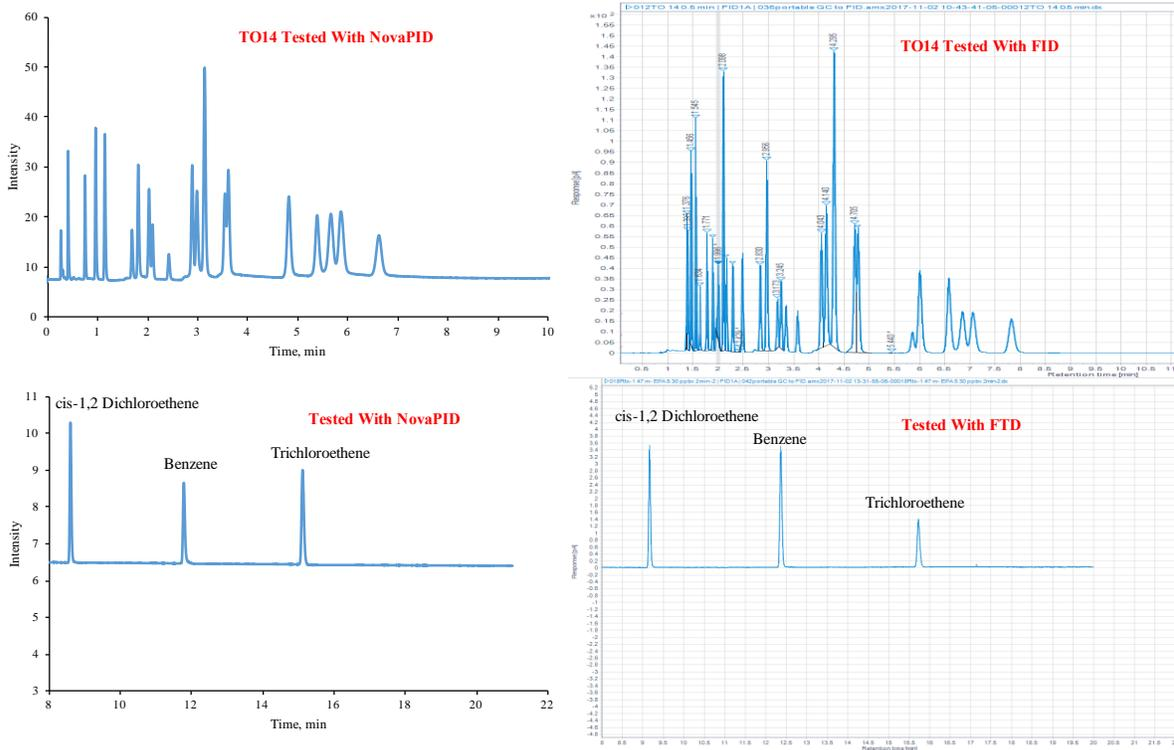
**Figure 5. Sample Chromatograms when using the NovaPID and a commercial FID, respectively. Injected sample included TO14 and a three-compound mixture. Both the NovaPID and the FID were installed at the outlet of NovaTest P100 separately for the test.**
