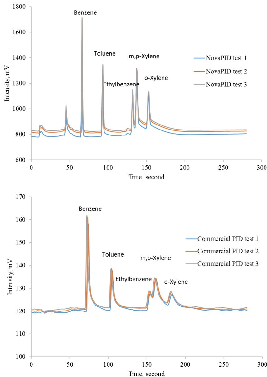
**Figure 4. BTEX tests using NovaPID and Commercial PID connected to NovaTest P100 compact GC. BTEX concentration: 1 ppm; Sampling time 0.2 min; Carrier gas flow rate: 2.2 ml/min.**
