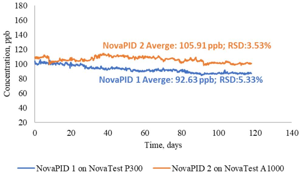
Figure 3. NovaPID aging test on NovaTest devices. Test time: 117 days
