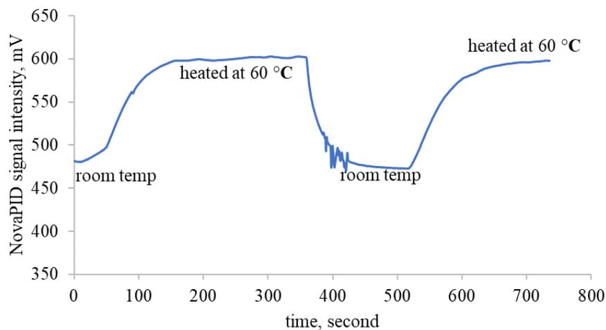
**Figure 2. NovaPID signal intensity when using at room temperature and heated at 60 °C**
