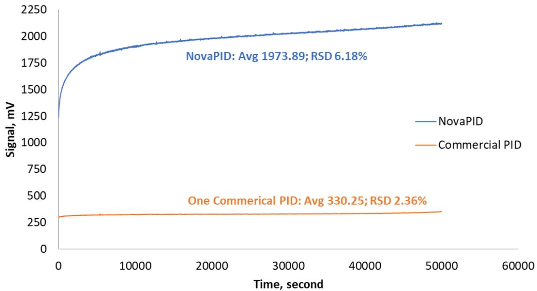
**Figure 1. PID aging test with 1 ppm BTEX**
