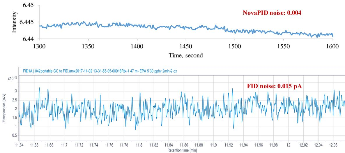
**Figure 6. The noise level of NovaPID and FID**
